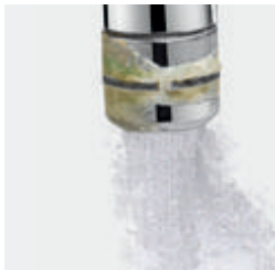
Scale build-up on aerator causes splashing
